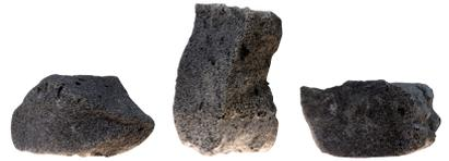
Let's talk about **GEOMATERIALS Foam Glass**. It is a building material for floor structures that saves energy, is light and load bearing, has thermal insulation properties and contributes to a comfortable indoor climate. A building material that is both economically and environmentally sound.
