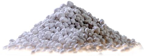
**GEOMATERIALS Expanded Glass** is formed of lightweight beads to banish cold, damp, and noise. This is a building material that is light as a feather, moisture-resistant, dimensionally stable (no settlement of the bound fill) and resistant to aging. Moreover, it is ideal as a loose or bound thermally insulating fill.
